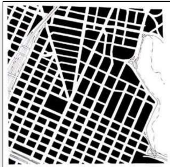
A grid network provides for continuity throughout the circulation system Source: www.tfhr.gov
